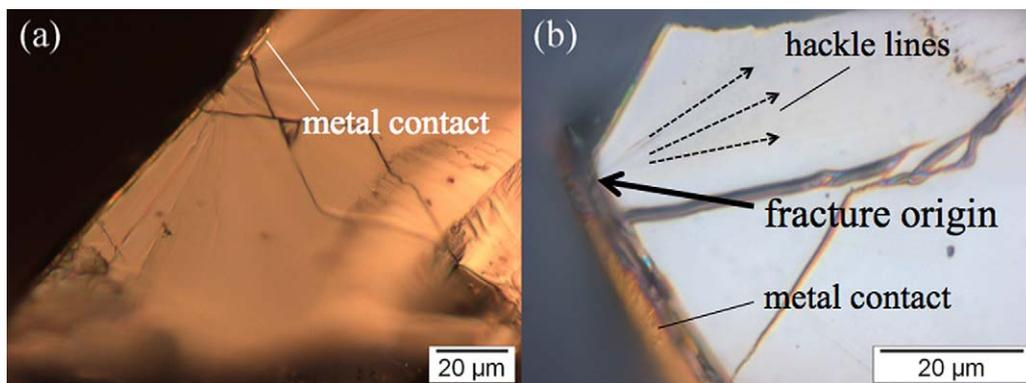
Fig. 7. (a) and (b) Microscopic images of the fracture surface of a Si chip that failed during metal-side B3B testing. Pictures are represented with increasing magnification (50 $\times$ , 100 $\times$ ) on either side of the fracture plane. Fracture originated in silicon in proximity of the metal–silicon interface. In (b) the direction of hackle lines allows to identify the region where the critical flaw was present.
