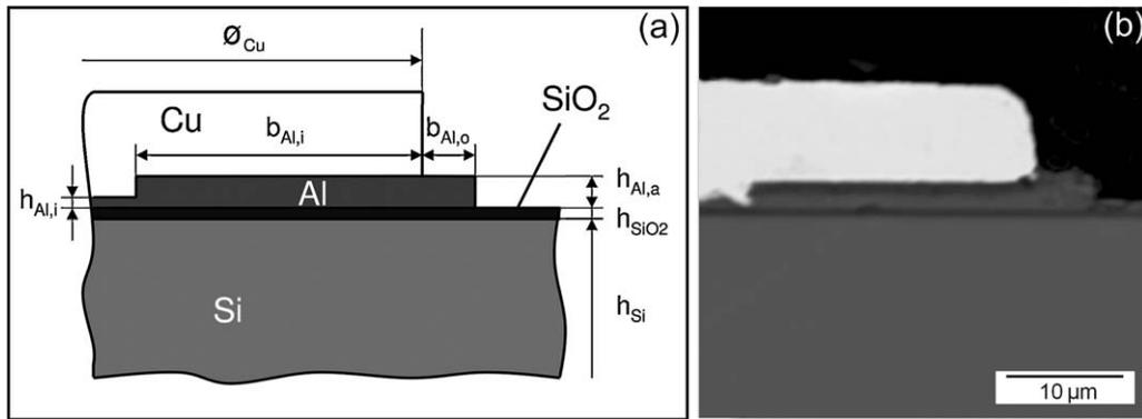
Fig. 2. (a) Description of the geometry adopted for FE sub-modelling of the metal-silicon interface. (b) SEM picture of the edge of the central metal contact on the patterned side of Si-chips.
