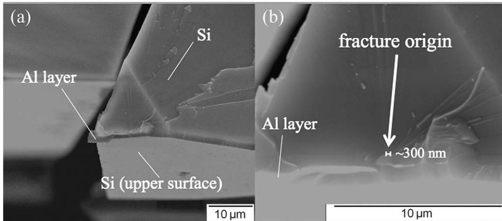
Fig. 9. SEM images of the fracture surface of a Si chip that failed during metal-side B3B testing. Magnification: (a) 5000 $\times$ , (b) 20000 $\times$ . Fracture originated in silicon in proximity of the Al–silicon interface. The size of the critical defect is  $\approx$ 300 nm.
