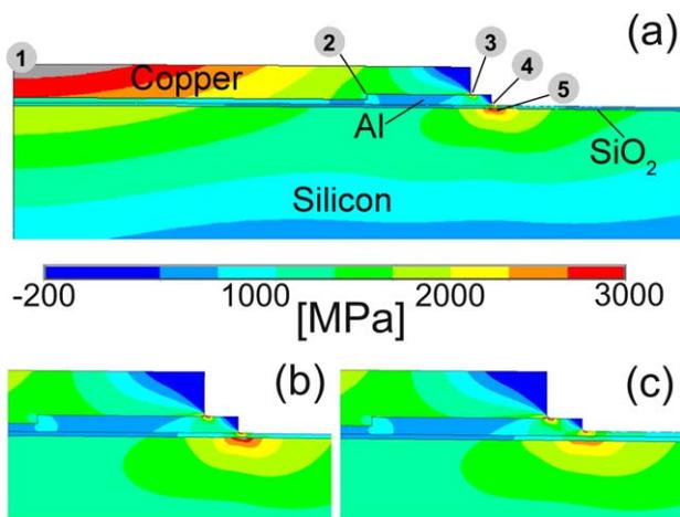
Fig. 10. (a) Location of the critical points in the neighbourhood of Cu contacts and FE results displaying the effect of a metal-side B3B test on the patterned side of Si-chips. (b) and (c) Magnified view of the electrode edges subjected to tensile stress concentration, in the absence or the presence of Al-interconnects, respectively. The same colour scale applies for all the displayed results.
