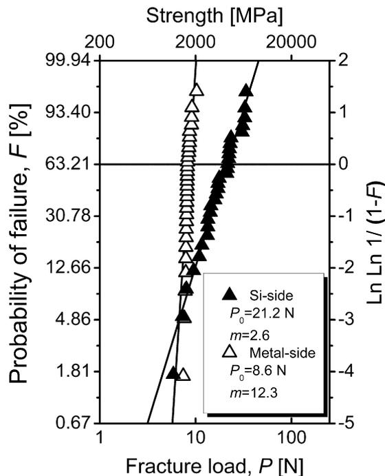
Fig. 4. Fracture load vs. probability of failure plot for Si-chips, obtained with B3B flexure tests. The obtained values of characteristic fracture load for both Si-side ( $P_0 = 21.2 \text{ N}$ ;  $m = 2.6$ ) and metal-side ( $P_0 = 8.6 \text{ N}$ ,  $m = 12.3$ ) samples are explicitly reported. The equivalent strength (in MPa) as calculated by Eq. (1) is also indicated.
