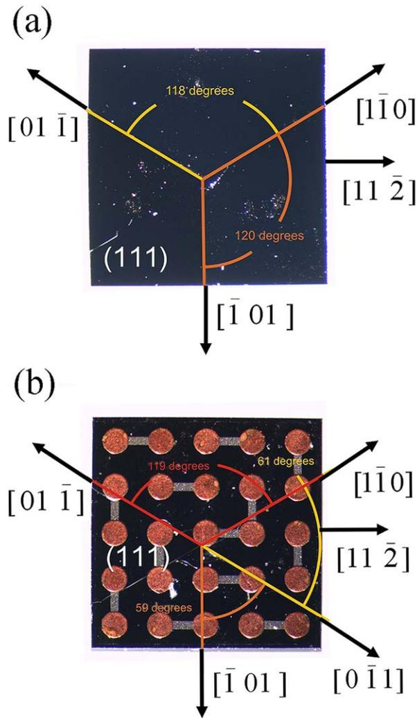
Fig. 5. Preferred fracture directions for (a) Si-side and (b) metal-side specimens tested with the B3B method. Fracture always involves the low-energy  $\{110\}$  planes intersecting the  $(111)$  plane.
