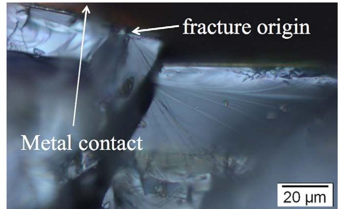
Fig. 8. Microscopic image of the fracture surface of a Si chip that failed during metal-side B3B testing (magnification: 50 $\times$ ). Fracture originated in silicon in proximity of the metal–silicon interface.
