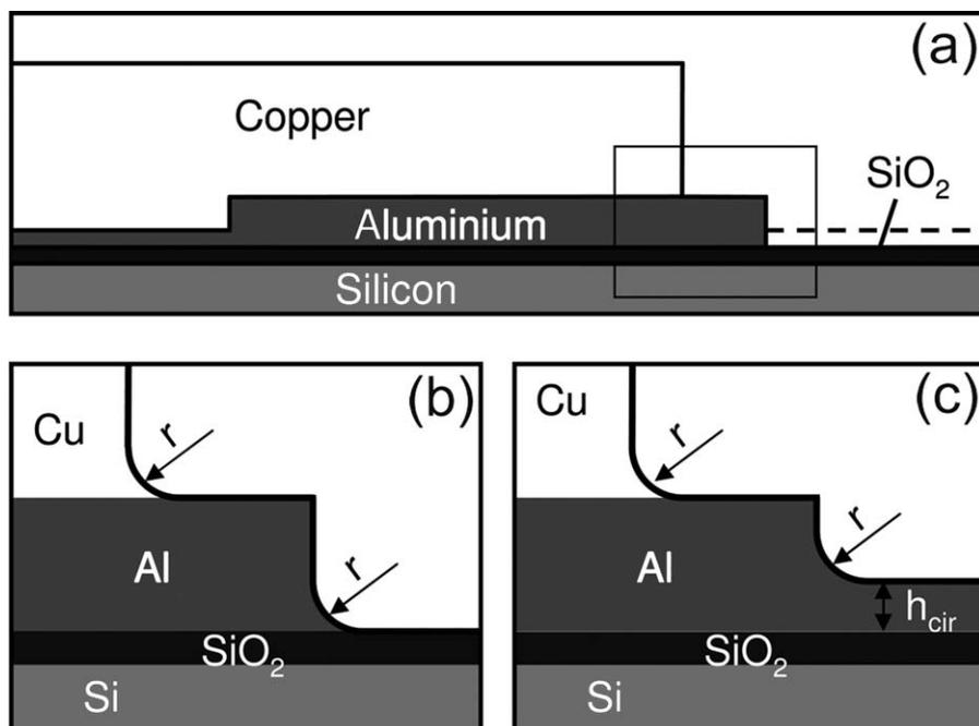
Fig. 3. Description of the two different geometries considered for sub-modelling of the electrode edge. (a) Overall view of the electrode area. (b) and (c) Layer edges in the absence or the presence of Al-interconnects, respectively.
